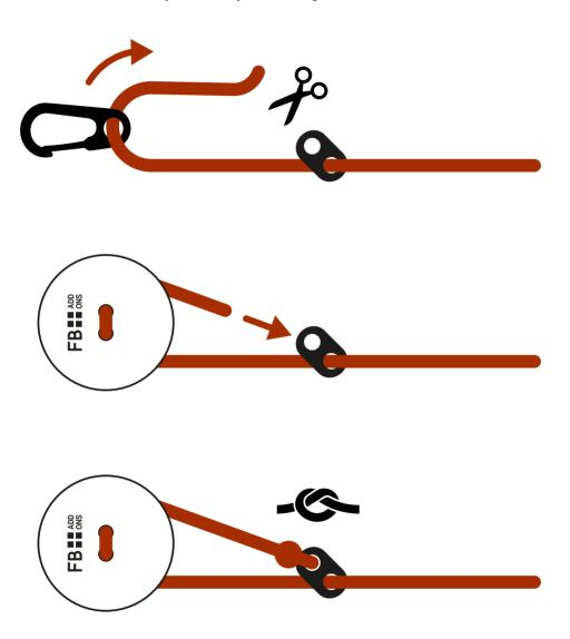
To replace the carabiner, untie or cut the harness cord close to the sliding lock on the side that holds the carabiner. Replace the carabiner with the Harness Button and tie the harness cord back to the sliding lock.
